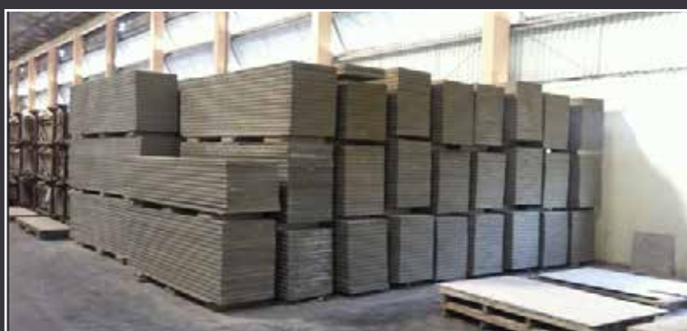
Always keep the tongue side of the Vpanel facing the sky/roof i.e. on the top side to avoid the damage to the tongue.
